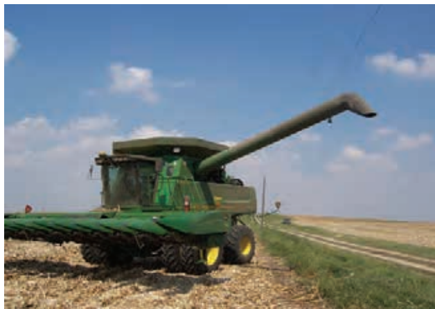
Always keep equipment at least 10 feet away from power lines—above, below and to the side—a 360-degree rule.
